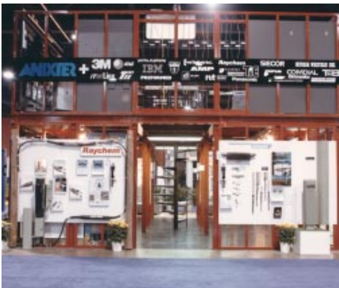
Above: Lightweight, easy to assemble two story trade show exhibit structure is fabricated of EXTREN®.
