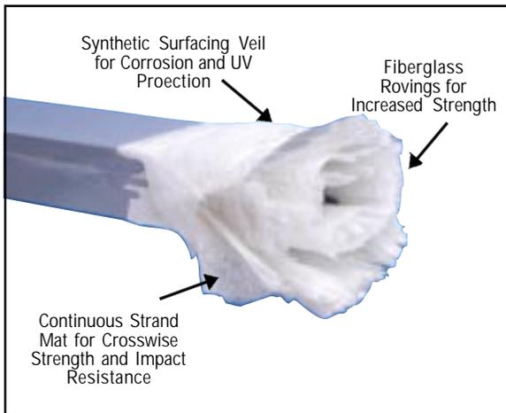
*EXTREN® is a proprietary combination of fiberglass reinforcements and thermosetting polyester or vinyl ester resin systems. It is produced in more than 100 standard shapes*
