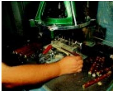
Custom electrical crossbars are pultruded with a high temperature epoxy resin, post cured, and cut to length. A multiple spindle drill maintains the tight hole tolerances required.
