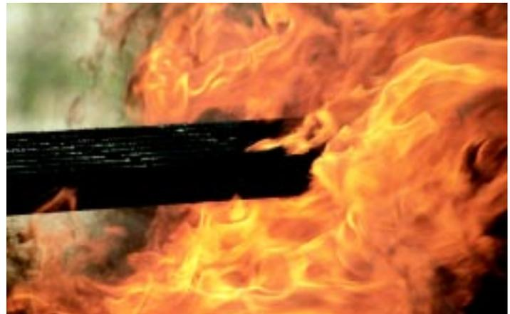
*Strongwell is the leader in the research and development of pultruding with phenolic resins. A dramatic innovation for markets where fire safety is a major concern, DURAGRID® Phenolic Grating withstood temperatures over 1700° F for one hour during testing per USCG 46 CFR CH. 1.*
