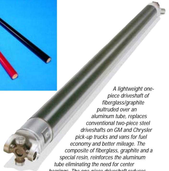
*A lightweight one-piece driveshaft of fiberglass/graphite pultruded over an aluminum tube, replaces conventional two-piece steel driveshafts on GM and Chrysler pick-up trucks and vans for fuel economy and better mileage. The composite of fiberglass, graphite and a special resin, reinforces the aluminum tube eliminating the need for center bearings. The one-piece driveshaft reduces assembly time, inventory costs, powertrain noise and vibration, and maintenance.*
