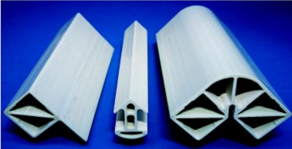
Three highly complex pultruded profiles were developed for a communications shelter on the US Army's High Mobility Multi-purpose Wheeled Vehicle (HMMWV). Designed with special reinforcements and close dimensional tolerances, the custom profiles exhibited numerous production challenges.
