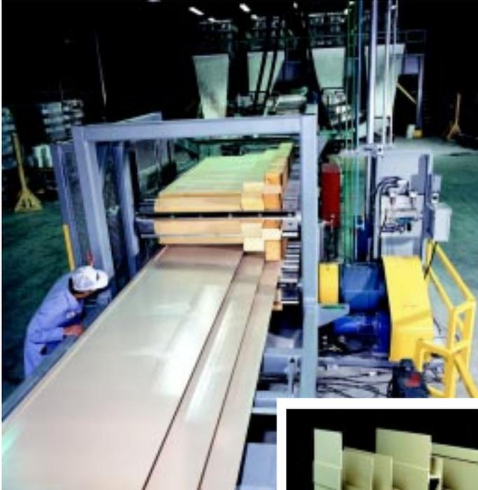
Seven interlocking components form the structure of an all fiberglass cooling tower. A custom pultrusion machine (one of the largest in the world) was specially designed to pultrude the two largest components, hollow profiles nearly 4' wide and up to 10" deep.
